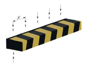
4. When everything is properly adjusted, screw (maximum tightening torque 2 Nm) the screws supplied into the plastic rail (groove) at an even distance "B" (not larger than 200 mm). Check, if all installation components are firmly joined.
